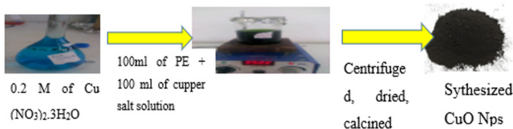
Fig. 3. General procedure for the biosynthesis of copper oxide nanoparticles using M. stenopetala extract
