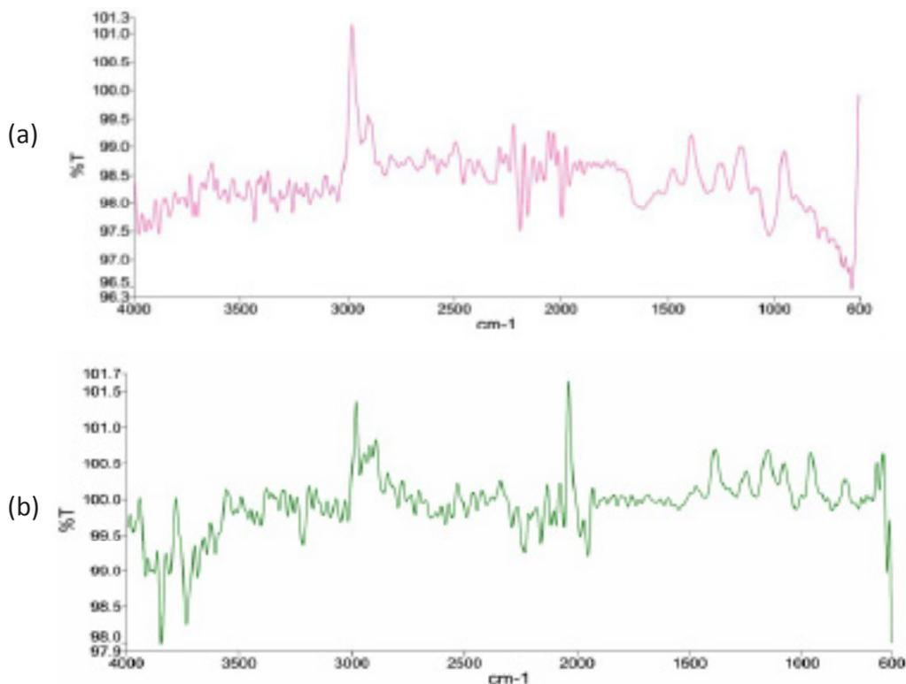
Fig 3. FT-IR spectra of (a) AgNPs, and (b) Li-AgNPs
