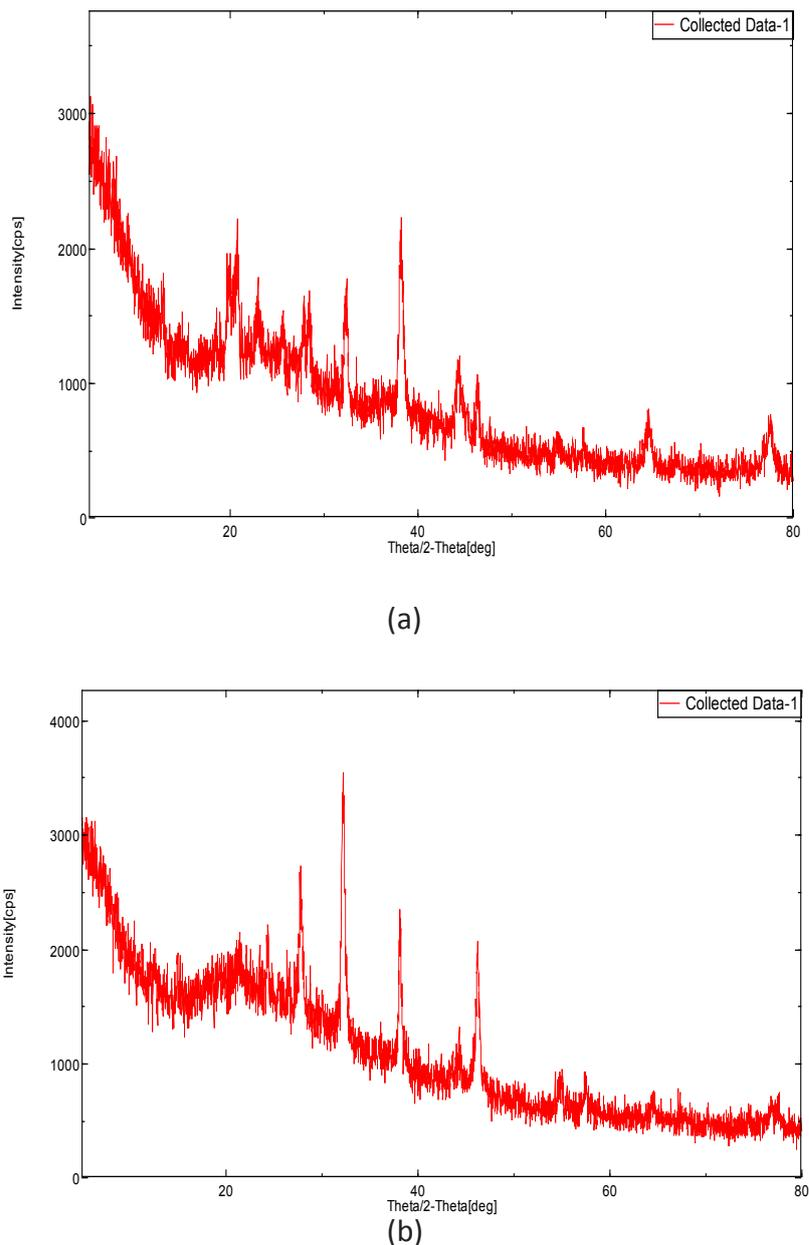
Fig 4. XRD analysis of (a) AgNPs, and (b) Li-AgNPs
