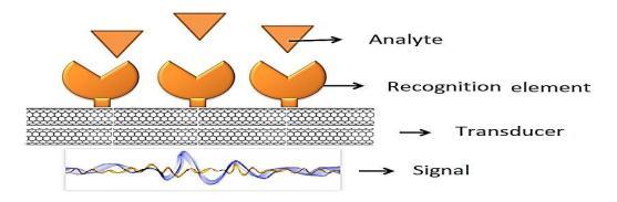
Figure 1. Schematic presentation of a biosensor.
