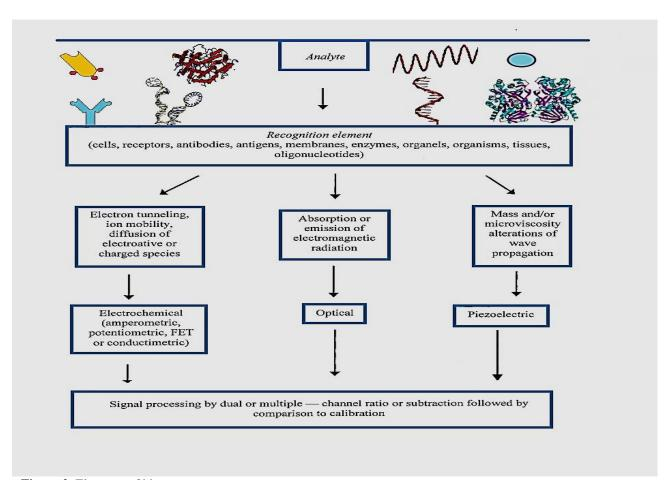
Figure 2. Elements of biosensors
