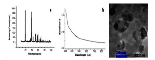
Fig. 1. The physicochemical properties of MgO nanoparticles. 1(a), X-ray diffraction pattern. 1(b) the visible spectrum - ultraviolet. 1(c) TEM image
