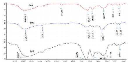
Fig. 2. FTIR spectra of (a) chitosan (b) CNPs, and (c) O. basilicum leaf extract
