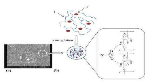
Scheme. 1. Proposed mechanism to form of chitosan nanoparticles by ionotropic gelation: (a) SEM image of the biosynthesized nanoparticle, (b) schematic illustration of the chitosan-anion complex. 1 chitosan and 2 negatively charged functional groups of *O. basilicum* leaf extract such as coo<sup>-</sup>
