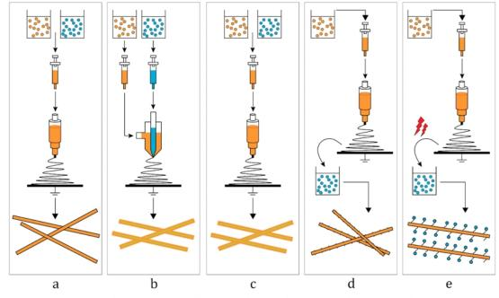
Fig. 2. Schematic picture of different methods of drug incorporation into nanofibers a. blending; b. coaxial electrospinning; c. emulsion electrospinning; d. surface modification (physical adsorption); e. surface modification (chemical immobilization)
