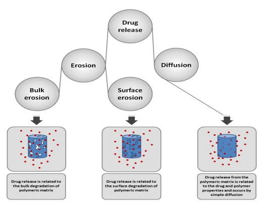
Fig. 3. Schematic drug release manners from electrospun nanofibers
