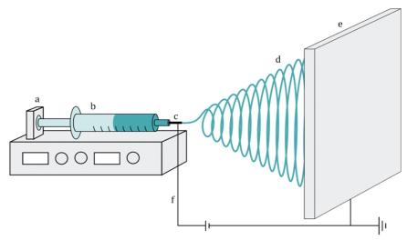
Fig. 1. Schematic picture of a typical electrospinning setup a.syringe pump; b.syringe containing polymer solution; c. spinneret needle; d. Nanofibers formation; e. collector plate; f. high-voltage supply
