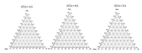
Fig 1. Pseudo-ternary phase diagrams for first microemulsion formulation (Tween 80-Glycerin-Sesame oil-water)
